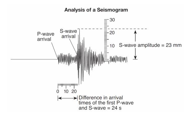
The diagram below represents how the earthquake's magnitude is determined by drawing a line connecting the difference in arrival times of the P-wave and the S-wave, and the S-wave amplitude.
